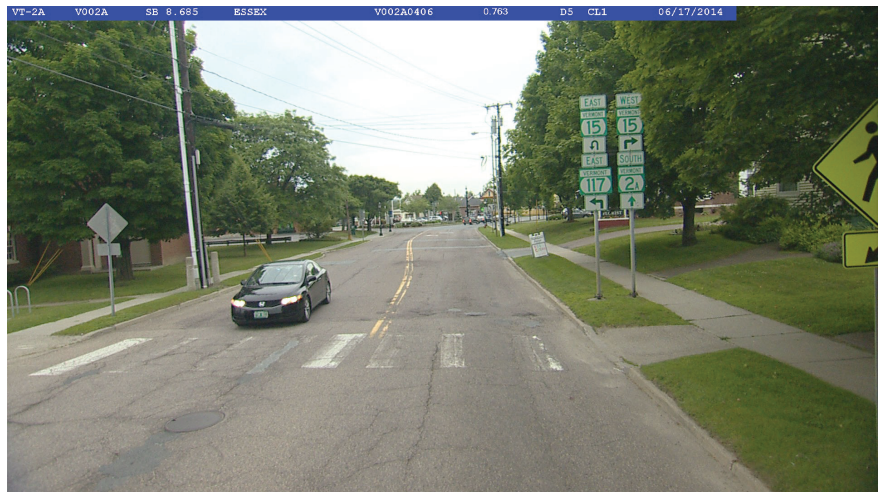
Figure 1. An example of a sign assembly containing multiple signs of similar appearance. All of the signs on the assembly have a green and white appearance, so it is difficult for a model to distinguish between them. There are two signs containing the word “East” which appear essentially identical. There are also two signs with the text “Vermont 15”. The arrow in the bottom left is a mirrored version of the arrow in the middle right. Since these signs contain so many similar characteristics, and in some cases are nearly identical, it is extremely challenging to create a geo-localization model that separately geo-localizes these signs.
