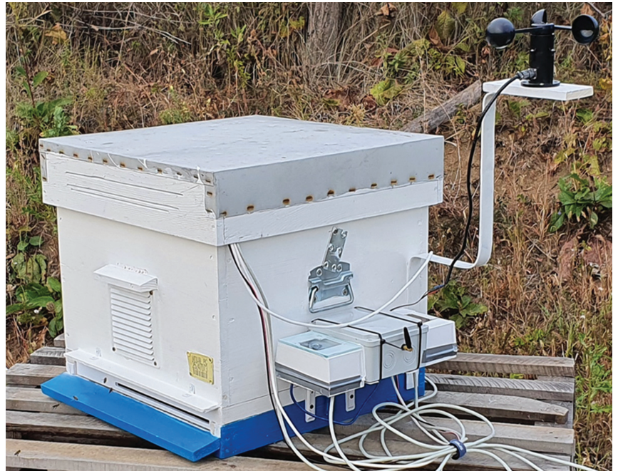
Figure 2. Experimental hive setup with sensor electronics.
