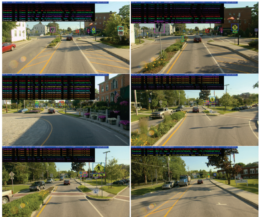
Figure 8. Sample images and detections from the ARTSv2 dataset. Images contain a variety of sign types, often clustered very close together, which makes for challenging geo-localization. Each box around each sign represents a separate detection from GPS-RetinaNet. The color of the box represents which tracklet the detection has been assigned to by the multi-object tracker. Since a tracklet is a list of signs predicted to be the same, re-occurrences of the same sign in multiple images should have the same color box around it.
