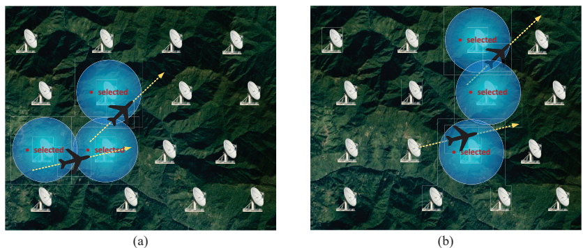
Figure 1. Illustration of dynamic selection of a fixed number of sensors for MTT: (a) At time k ; (b) At time k + 1 . It is assumed that three sensors are selected at each time step, and the blue circles show the coverage areas of the selected sensors.
