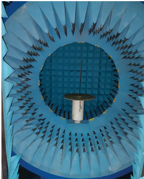
Figure 20. Fabricated antenna inside the anechoic chamber for the radiation pattern measurement.
