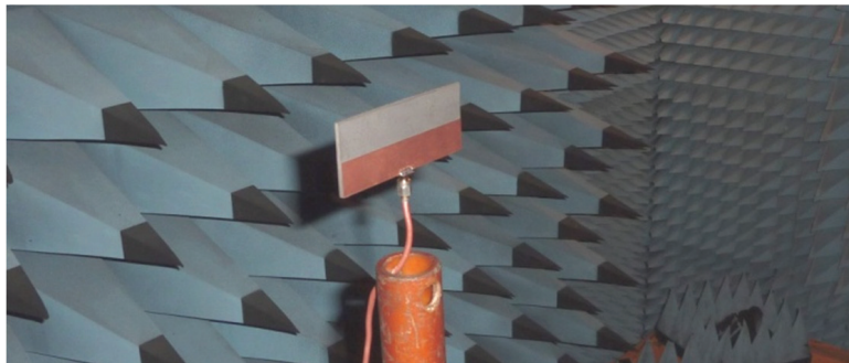
Figure 5. Longer variant of four-element antenna array in anechoic chamber during measurements.
