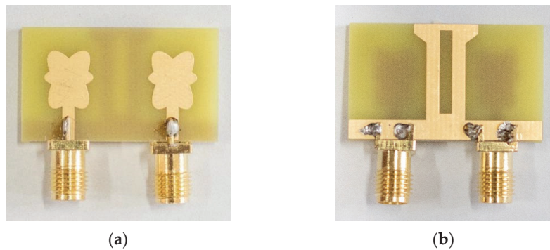
Figure 2. Fabricated prototype of the proposed dual-port, flower-shaped UWB-MIMO antenna: (a) front view, (b) back view.
