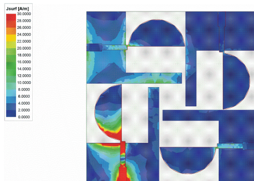
Figure 3. Surface current distribution at 6.5 GHz for ant3.
