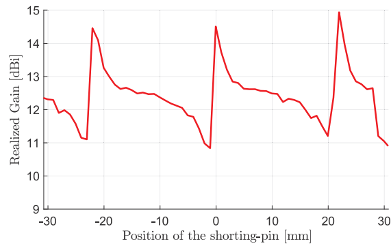
Figure 8. Gain of four-element antenna vs. position of shorting pin along feed patch.
