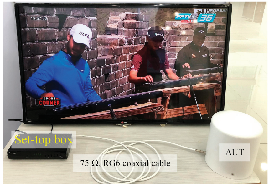
Figure 24. The experimental setup for the reception test in actual use.
