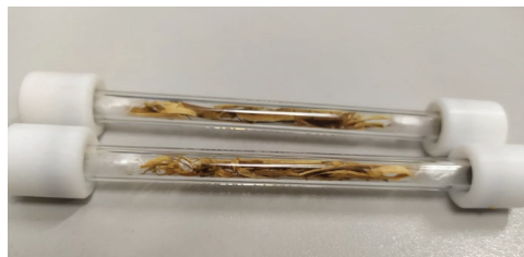
Figure 4. Chips planed from wooden floor staves coated with bituminous products, ready for thermal desorption tests.
