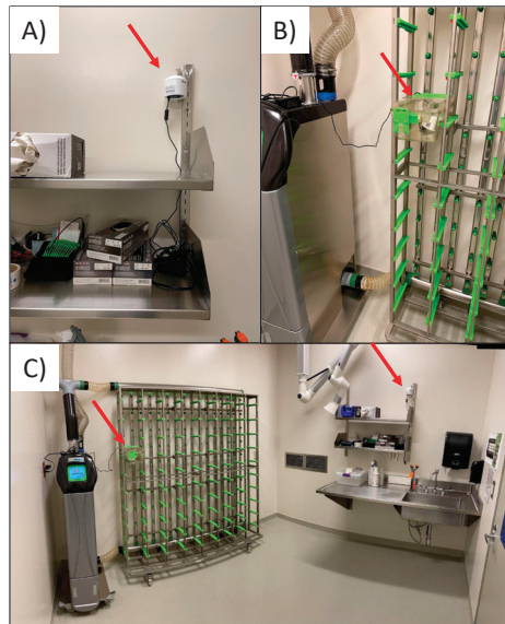
Figure 2. Placement of indoor sensors including (A); indoor wall location, (B); indoor HEPA cage location, and (C); room where both indoor sensors were located.
