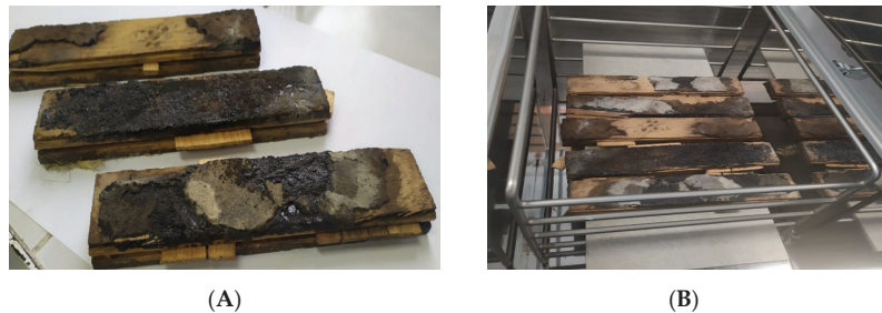
Figure 3. (A) Wooden floor staves coated with bitumen, collected from the renovated office room (B) The same floor staves placed in the emission chamber.
