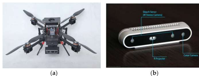
Figure 3. Data acquisition equipment of the study. (a) FEISI X450 UAV; (b) Intel d435i binocular camera.
