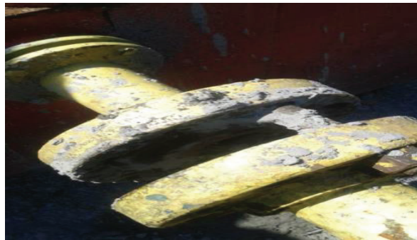
Figure 1. Crust of oil installations (photo provided by Stefan Petrache) [8].
