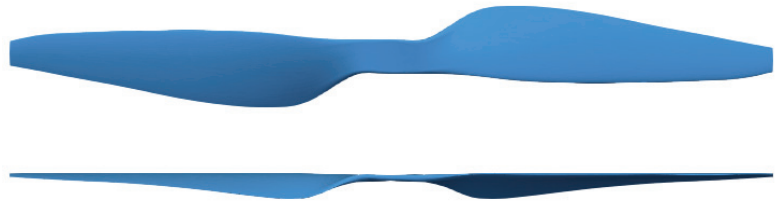
Figure 4. Top view ( top ) and front view ( bottom ) of the computational 3D rotor geometry for a pitch of 9.2".
