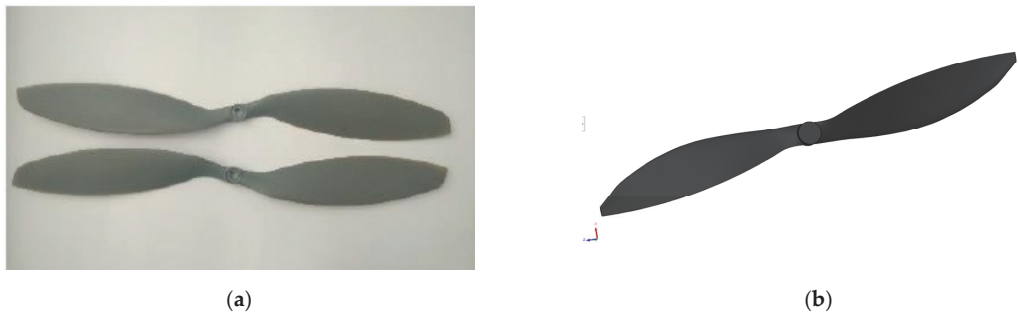
Figure 7. APC1047SF air rotor: (a) physical map; (b) model diagram.
