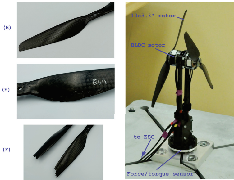
Figure 1. Samples of rotors used in fault detection experiments and overview of the propulsion test rig.
