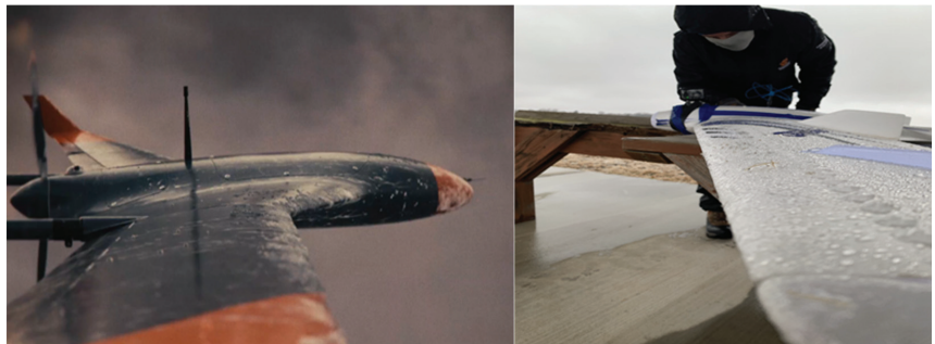
Figure 1. Ice accretion on fixed-wing UAV [13,14].
