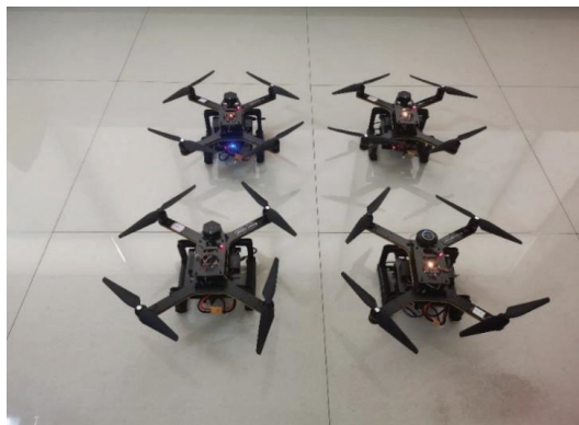
Figure 3. UAV swarms for carrying real-time target detection and sensing systems.
