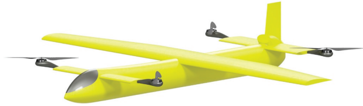
Figure 11. Three-dimensional model of the VTOL lane with a transverse arm configuration.
