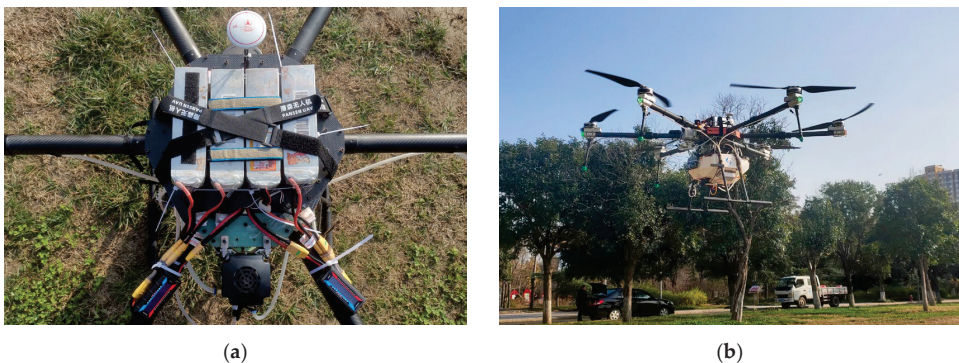
Figure 14. The hovering time test of the ecological plant protection UAV: (a) install the power meter; (b) the UAV stays in hover.
