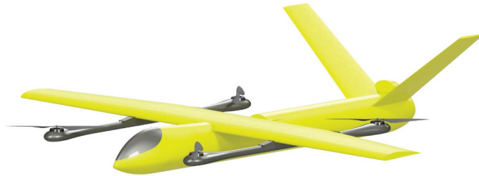
Figure 7. Three-dimensional model of the VTOL plane with a quad-plane configuration.
