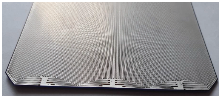
Figure 7. Rear surface of Maxeon Ne3 with visible connectors in the lower part.
