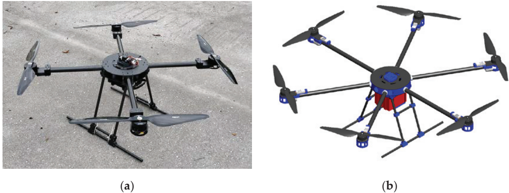
Figure 1. Multirotor UAV platform: (a) quadrotor heavy-lift prototype; (b) hexarotor 3D model.
