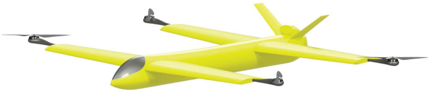
Figure 9. Three-dimensional model of the VTOL plane with the tandem wing configuration.
