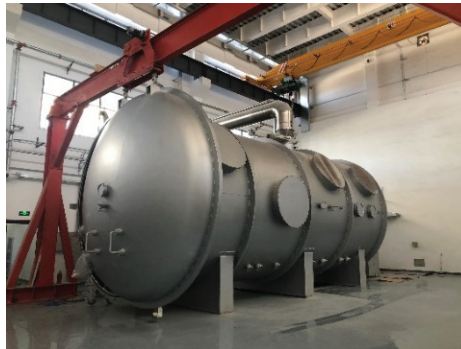
Figure 11. A vacuum chamber simulating the atmospheric environment of Mars.
