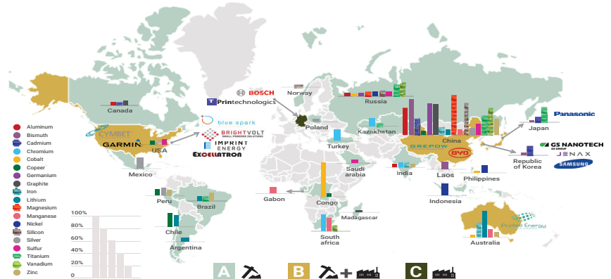
Figure 5. Geographical distribution of mineral resources vs. battery manufacturing companies. (A) Countries with mineral resources, (B) countries with mineral resources and manufacturing companies, and (C) manufacturing countries. Note: the length of the bar indicates the relative fraction of the total production. Graph constructed by the authors. Data from US Geological Survey, Mineral Commodity Summaries 2020.
