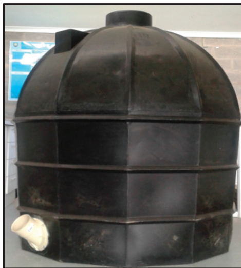
Figure 1. Fabricated high-density polyethylene biogas digester.
