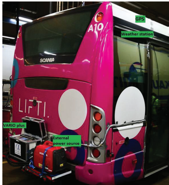
Figure 1. Measurement system set-up.
