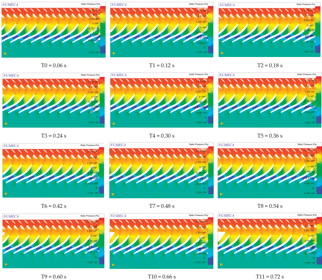
Figure 12. Pressure distribution on the flow surface inside the turbine and guide vanes at 50% blade height under 80% operating conditions of the hydro-turbine.
