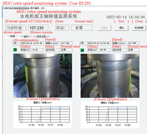
Figure 13. The experimental results of HGU rotor speed monitoring system.
