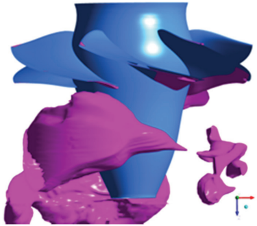
Figure 17. Iso-surface of 20% vapor volume fraction at OP2 in the runner domain.
