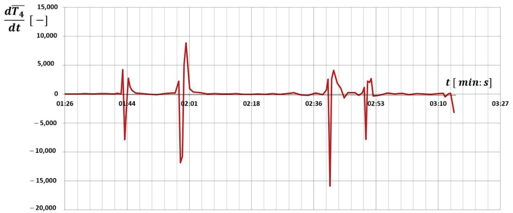
Figure 1. Temperature-change trend downstream of the jet engine turbine during an engine surge.
