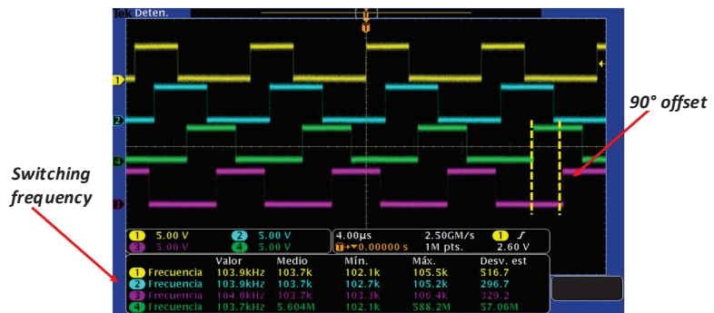
Figure 9. Commutation signals for phases with the corresponding 90^\circ phase shift and duty cycle (40%).
