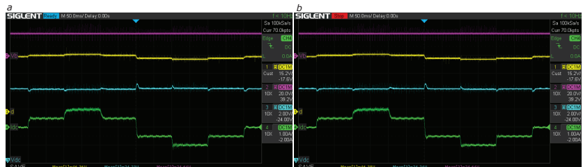
Figure 28. Bus regulation with v_b = 24 V and reference v_{dc_{ref}} = 24 V (unity gain mode) using adaptive LQG by (a) lookup table and (b) polynomial interpolation. Magenta: battery voltage v_b ; yellow: duty cycle d ; cyan: bus voltage v_{dc} ; green: bus current i_o .
