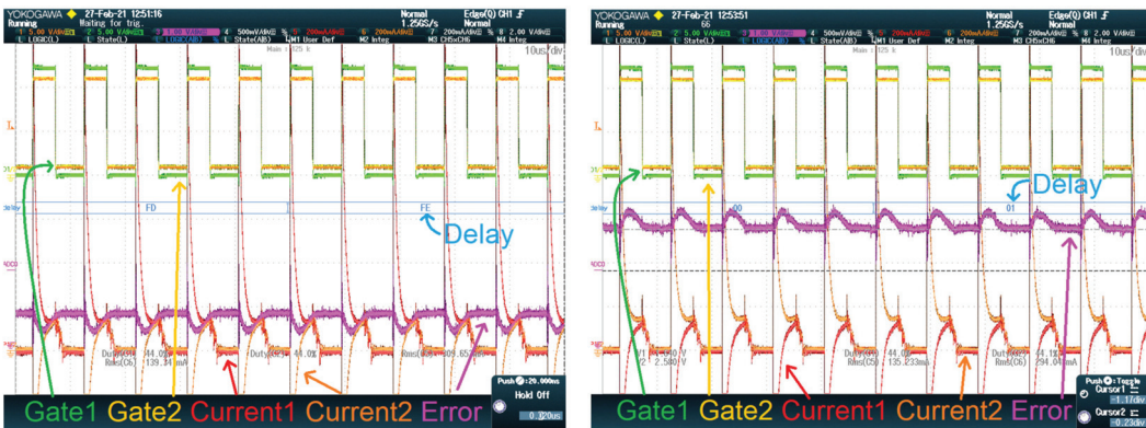
Figure 12. Fixed 62 ns timing error between the two sub-forwards: negative error (left) and positive error (right).
