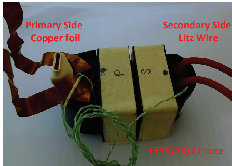
Figure 8. The 5 kW ferrite core (N87) high-frequency transformer prototype.
