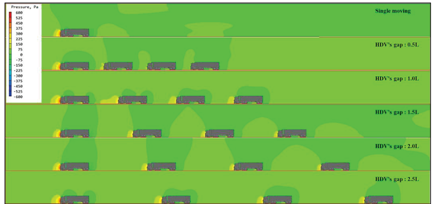
Figure 6. Comparison of the static pressure distribution with the change in the gap at 100 km/h.
