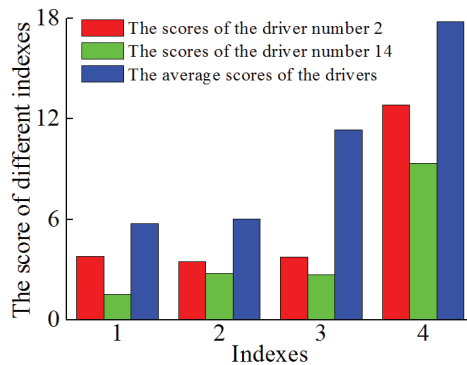
Figure 19. The comparison of scores for four indexes (numbers from 1 to 4 represent the number of rapid accelerations per 100 km, the number of sudden brakings per 100 km, the number of rapid turns per 100 km and the number of speeding occurrences during steering per 100 km, respectively).
