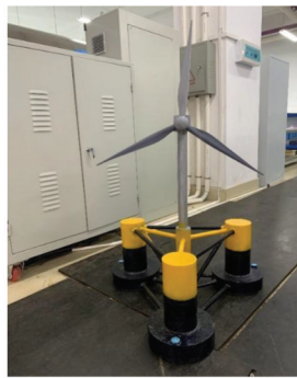
(a) Supported by OC4-DeepCwind platform.
