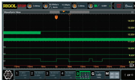
Figure 21. LED control triggered by sound detection circuit.
