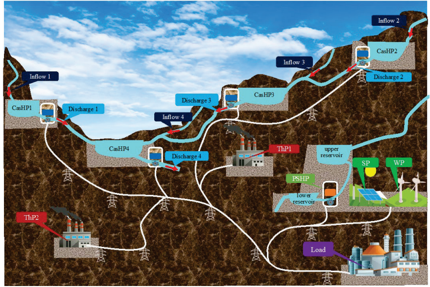
Figure 1. The structure of the considered hybrid system.
