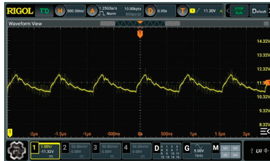
Figure 19. SW pin of LED driver circuit.
