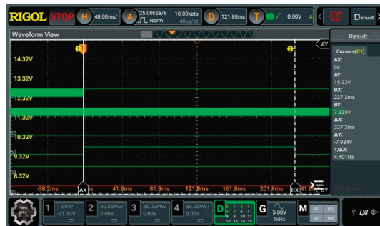
Figure 22. LED control triggered by PIR detection circuit.
