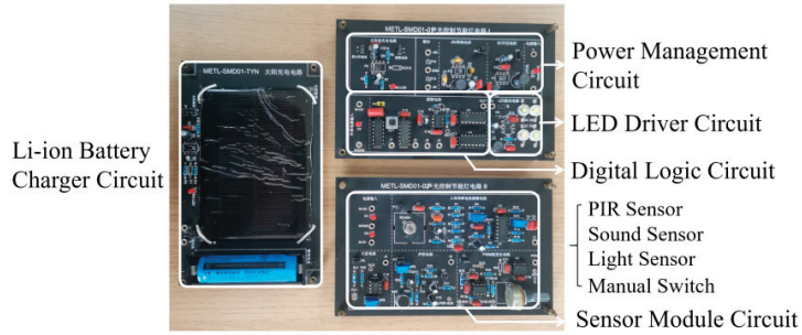
Figure 18. Testing platform of intelligent controller.
