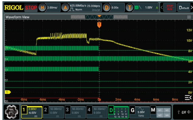
Figure 24. LED control triggered by light detection circuit.
