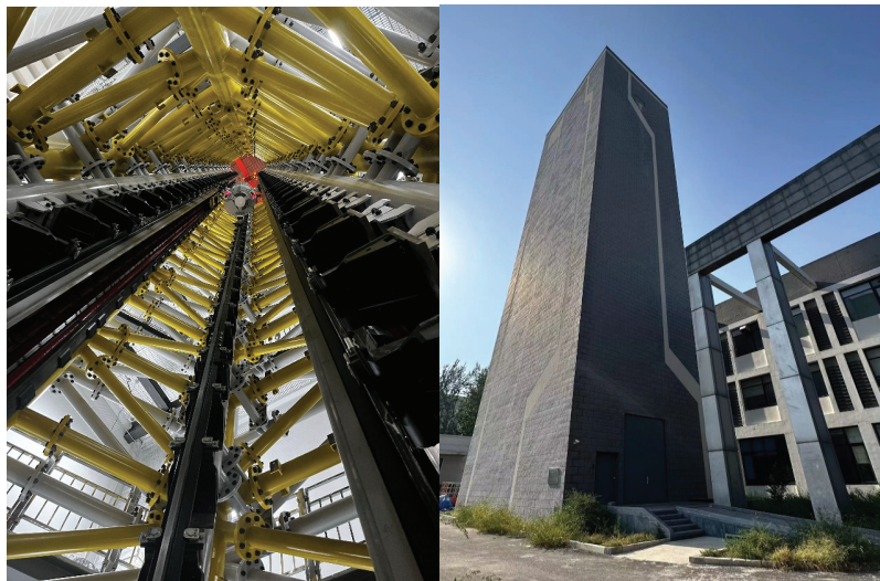
Figure 15. MEFEL experimental platform with vertical LIM.
