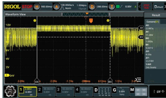
Figure 20. SW pin after starting the timing circuit.
