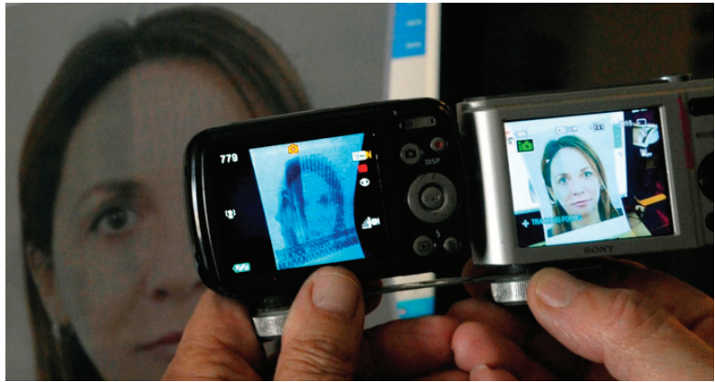
Figure 1. Print studied with a ZRGB camera (Z blockage at 1000 nm and in the visible spectrum; blockade at 400 nm).
