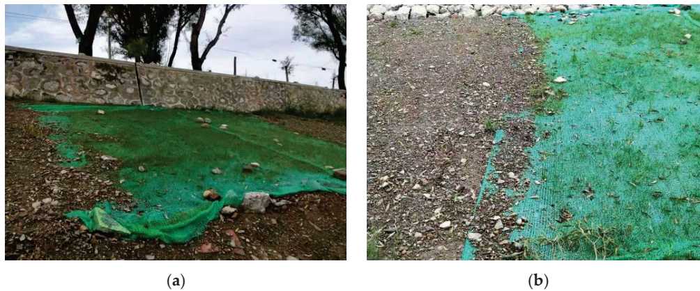
Figure 11. The condition of the slope under the impact of the rainfall on the 17th day after seeding. (a) vegetation observed above the blanket; (b) comparison of conditions of the treated and bare slopes.
