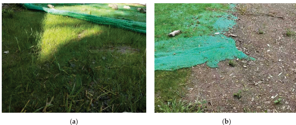
Figure 10. Vegetation growth at the 13rd day after seeding: (a) vegetation growth within the selected area; (b) comparison of the vegetation growth on the treated and bare slopes.
