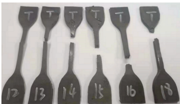
Figure 4. Damage diagram of type IV dumbbell specimen.
