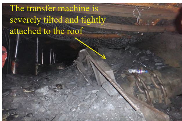
Figure 2. Photo of the tilting of the end transfer machine on the working face.
