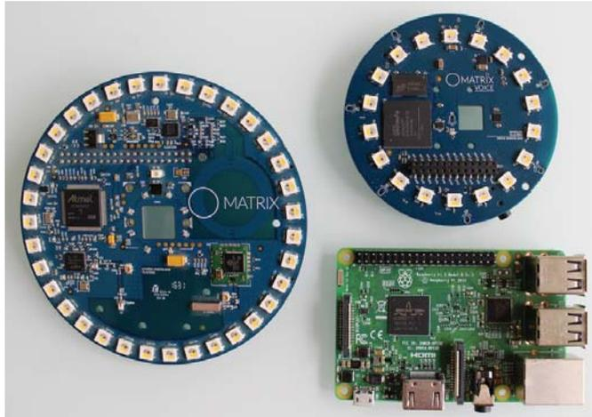
**Figure 3.** Examples of different development HAT for Raspberry Pi.
