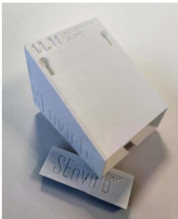
Figure 6. 3D printed enclosure.
