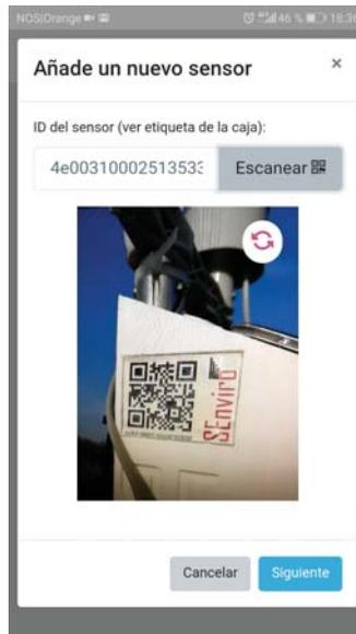
Figure 15. A screenshot of the *SEnviro* connect showing the wizard to claim nodes.
