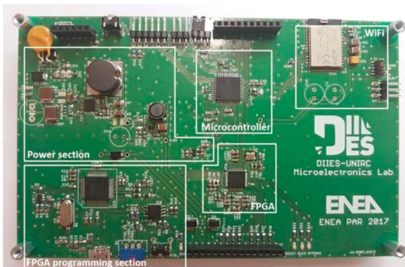
Figure 4. Main logic board top view.
