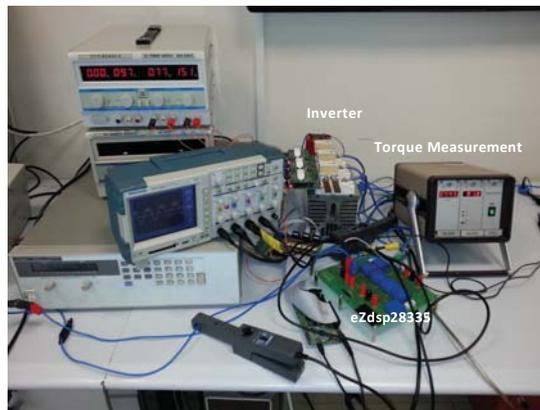
Figure 10. Experimental test-bed: inverter, DSP control unit and torque transducer.
