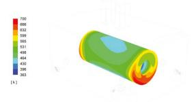
Figure 7. Temperature of the load surface after 2 h of the heat treatment—case 7.
