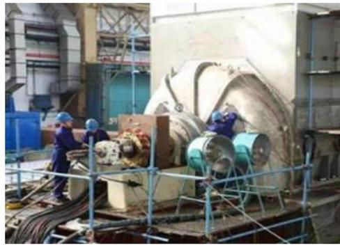
Figure 11. Temperature increase test system of the 300 Mvar synchronous condenser.
