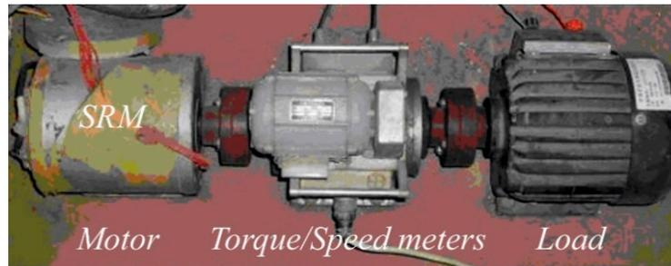
Figure 14. Measuring stand for determination of SRM-drive system properties.
