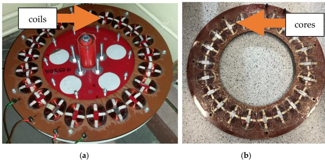
Figure 5. Stator discs; (a) coreless; (b) with cores.
