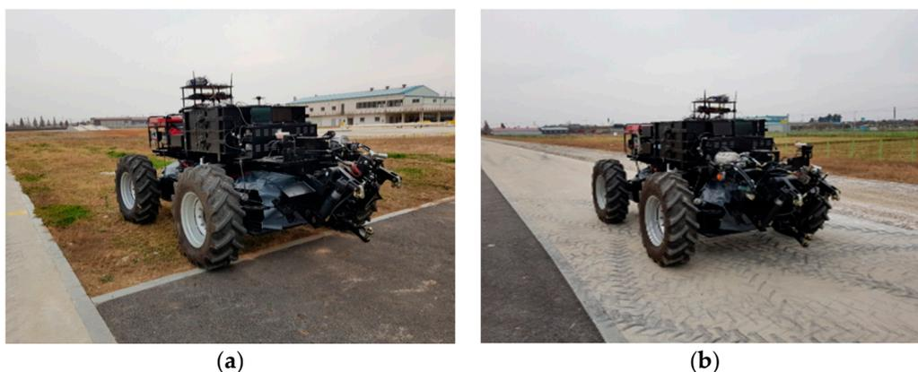
Figure 5. Photos of driving operation of electric AWD tractor under (a) off-road and (b) on-road conditions.
