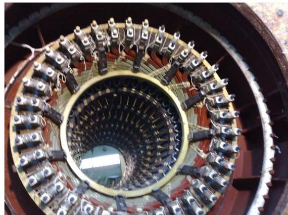
**Figure 1.** End structure of hydrogen-cooled turbo-generator prototype.
