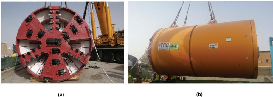
**Figure 5.** Trenchless technology equipment used in construction of storm sewer at the urban highway in study area shown in Figure 4. (a) cross-sectional view, (b) side view.
