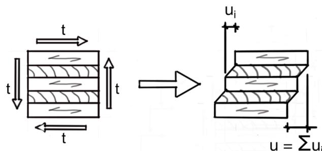
**Figure 4.** Shear deformations between layers of a cross laminated timber plate cross-section according to Mestek et al. [13], where  $t$  are the applied shear forces,  $u_i$  the resulting deformation of a transverse layer, and  $u$  the total deformation of the plate. Redrawn and adapted by the authors.
