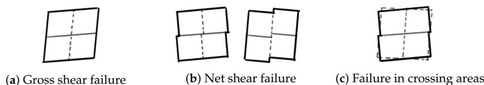
**Figure 5.** Failure modes of shear walls according to Danielsson et al. [14]. Redrawn and adapted by the authors.
