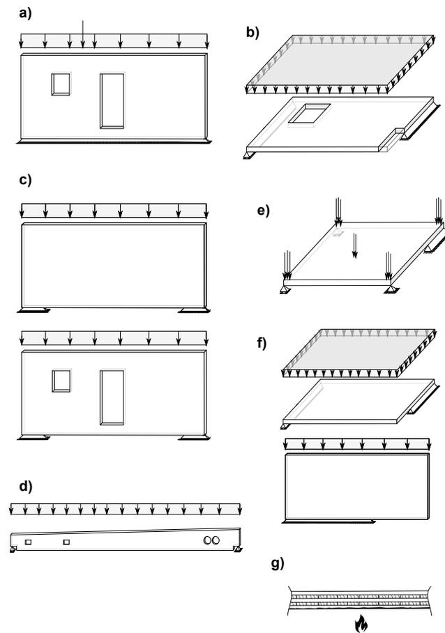
**Figure 13.** Challenging design situations for cross laminated timber (CLT): (a) openings in walls, (b) openings in floors, (c) deep CLT beams (with openings), (d) CLT beams (with openings), (e) point supports and concentrated loads, (f) cantilevers, (g) asymmetrical lay-ups.
