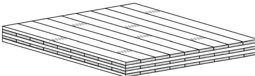
**Figure 1.** Example of a cross laminated timber panel [6].
