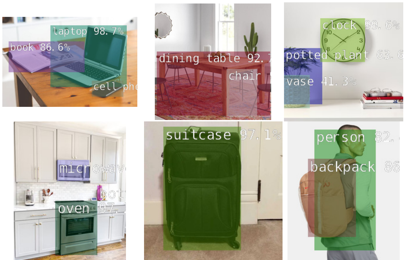
Figure 10. Several examples of object detection on test images. The object label, bounding box, and detection confidence levels are overlaid on the images.
