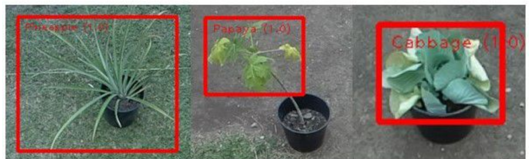
Figure 8. Object detection at an altitude of 2.5 m with Pi Camera.
