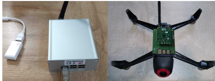
Figure 2. The IU880B node and the Raspberry IC880A platform (left). The IC880A platform mounted on the bottom of the drone (right).
