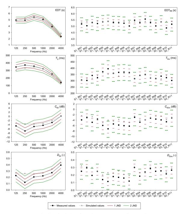
**Figure 6.** Measured and simulated values of several acoustic parameters (from top to bottom: EDT,  $T_S$ ,  $C_{80}$ , and  $D_{50}$ ): Spectral behaviour of the spatially averaged values (left column) and spectrally averaged values obtained at each source-receiver combination (right column). The values corresponding to 1 and 2 JND have been also included.
