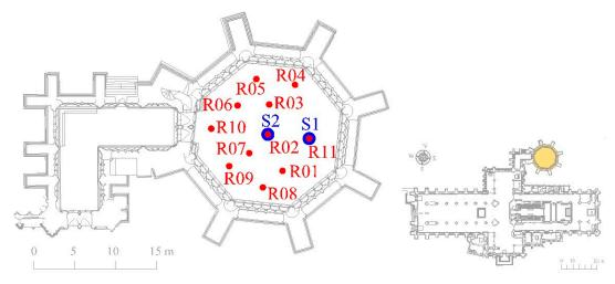
**Figure 1.** Floor plan of the York Minster's Chapter House with the source (S) and receiver (R) positions set for the acoustic measurements. The complete floor plan of the Minster is included for showing its location.
