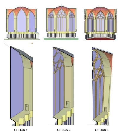
**Figure 5.** Acoustic model of the York Minster's Chapter House. Detail of the simplifications including the limestone canopies and the three options tested for the limestone clusters of shafts or nerves framing the stained glasses.
