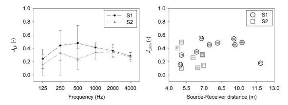
**Figure 9.** Spatially averaged values of the acoustic parameters as a function of frequency (left column)., and mid values as a function of source-receiver distance (right column).
