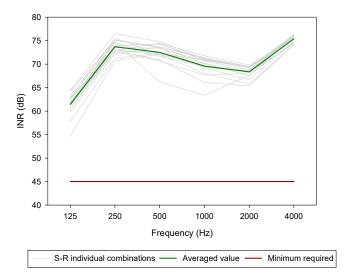
**Figure 4.** Impulse-to-noise ratio (INR) measured values obtained at each source-receiver combination characterised in the York Minster's Chapter House (grey lines) and the spatially averaged values (green line). The minimum value of INR required for a reliable calculation of  $T_{30}$  is also shown (red line).
