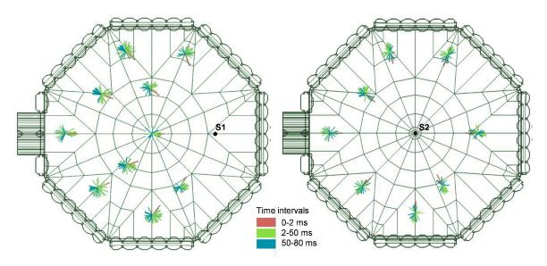
**Figure 10.** Representation of the early energy arriving at the receiver points (Iris plots, 2D XY plane, level range set to 40 dB with the direct sound level individually set as a reference (0dB)): front stage arrangement (left); and amphitheatre-like arrangement (right).
