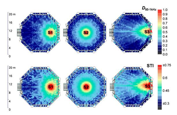
**Figure 12.** Simulated mappings of the  $D_{50}$  at 1 kHz (upper row) and STI (lower row) obtained for the different source positions. York Minster's Chapter House in its current state.
