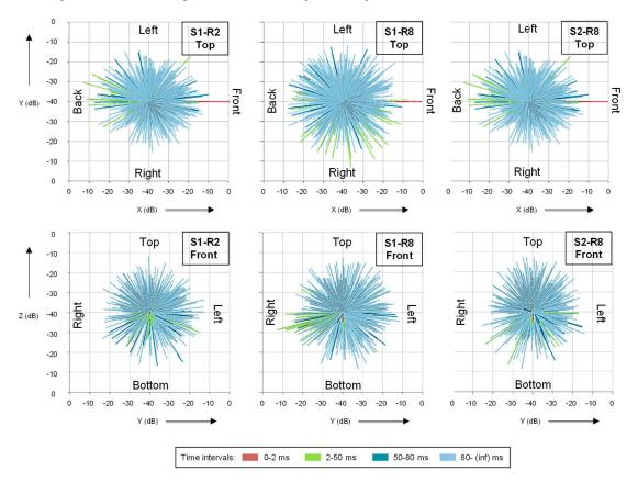
**Figure 11.** Representation of early and late energy arriving at selected S-R combinations (2D Iris plots, XY plane (upper row) and YZ plane (lower row), level range set to 40 dB with the direct sound level individually set as a reference (0 dB)).
