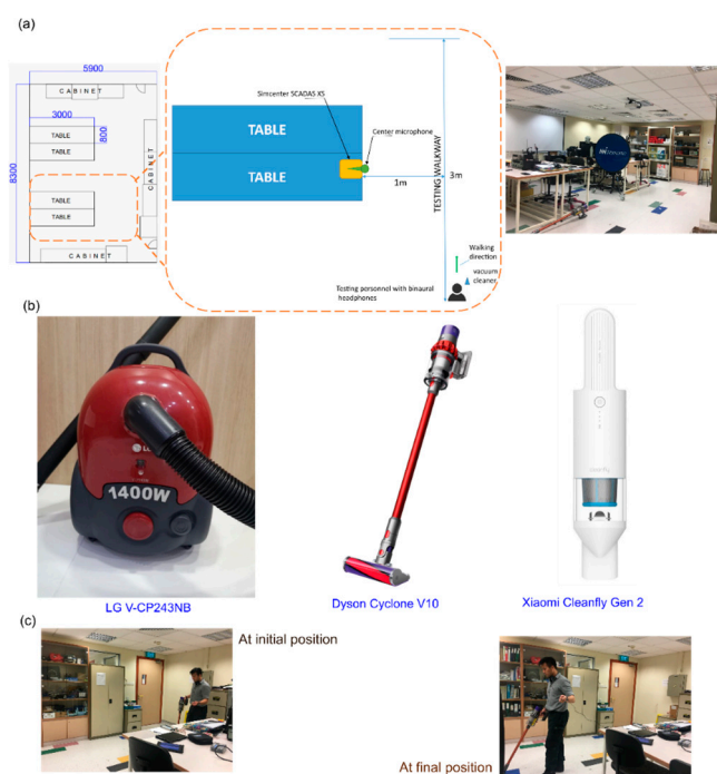
Figure 1. (a) Schematics of experimental setup plan. (b) Photographs of the three different vacuum cleaners. LG V-CP243NB (model type 1), Dyson Cyclone V10 (model type 2), and Xiaomi Cleanfly Gen2 (model type 3). (c) Photographs of the testing room displaying the vacuum cleaner positions.
