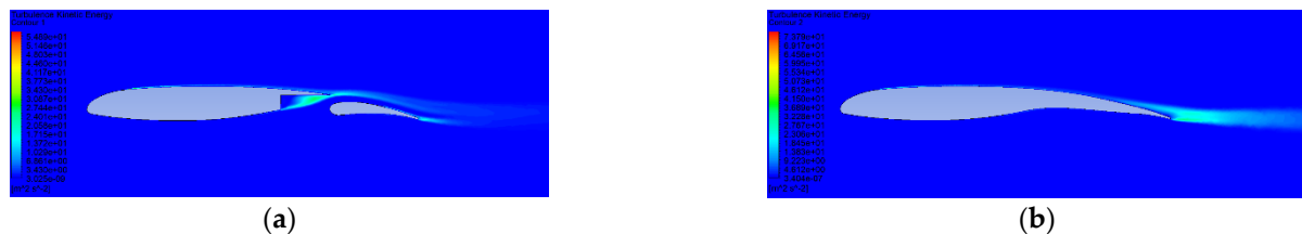
Figure 16. Turbulent kinetic energy (TKE) plot at 5° flap deflection: (a) conventional design; (b) morphed design.
