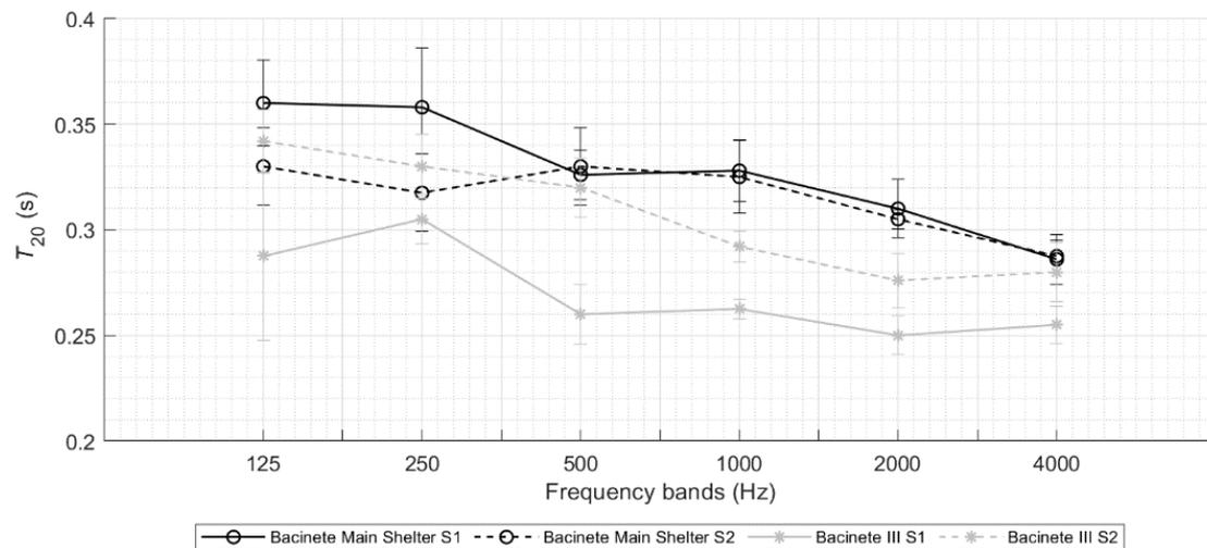
**Figure 6.** Reverberation time ( $T_{20}$ ) obtained in each shelter of the Bacinete rock art complex: Bacinete main shelter; Bacinete III. Spatially averaged values for each source location are represented at each frequency band.
