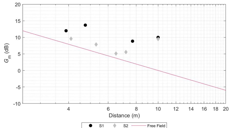
**Figure 9.** Sound strength,  $G_m$  (dB), spectrally averaged values calculated from the measured IR at Bacinete III. The theoretical free field propagation is represented by the red line.
