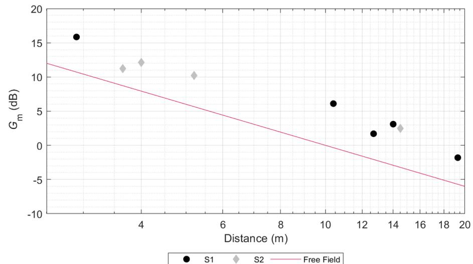
**Figure 8.** Sound strength,  $G_m$  (dB), spectrally averaged values calculated from the measured IR in the Bacinete main shelter. The theoretical free field propagation is represented by the red line.
