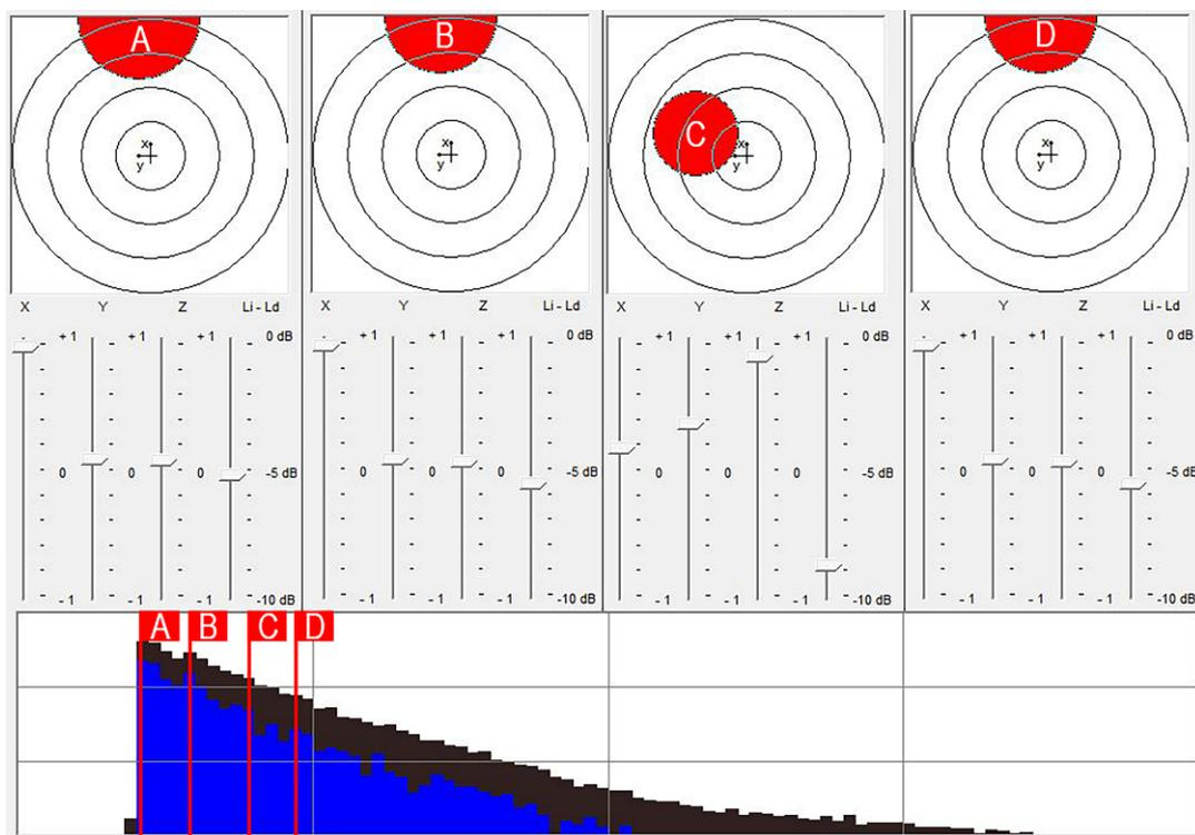
**Figure 7.** Example of the DOA analysis performed with the IRSpatial software tool. The 1st-order ambisonics impulse response corresponds to the S1-R4 combination in the Bacinete main shelter. Red dots show the DOA and the intensity of each group of reflections (A, B, C or D), the blue bars represent the sound intensity and the black bars the energy density of the signal.
