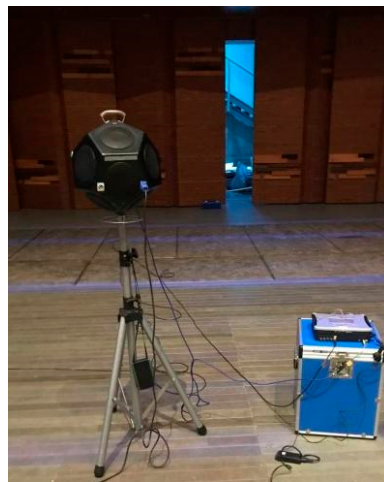
Figure 2. Omnidirectional source connected with the analyzer.
