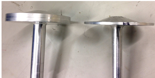
Figure 9. A picture showing the slim and large mushroom-shaped armatures. Although both are designed to withstand the mechanical stresses, one is flexible and prone to bending, while the other is more robust and stiffer.
