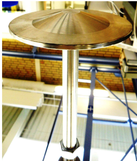
Figure 3. Mushroom-shaped conductive armature with threads on the stem's extremity to screw in a pull rod.
