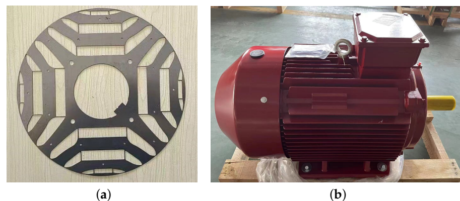
Figure 22. Manufactured prototype: (a) rotor core; (b) prototype assembly.
