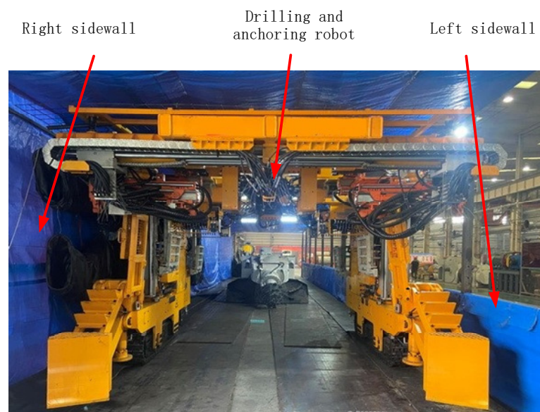
Figure 15. Drilling and anchoring robot test platform.
