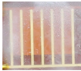
Figure 7. Physical picture of plasma actuator using water spray for ice-making.
