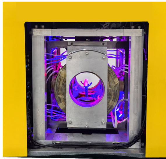
Figure 11. Physical Setup of the Wind Tunnel MSBS.
