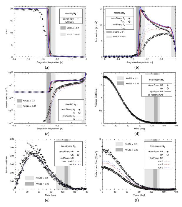
Figure 5. (a–c): Stagnation line profiles. CFD run 1: black lines, run 2: red lines, run 3: blue lines. (d–f): surface quantities around the cylinder. (a) Mach number; (b) temperature; (c) number density; (d) pressure coefficient; (e) skin-friction coefficient; (f) surface heat flux.
