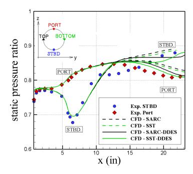
**Figure 10.** Turbulence model effects on CFD predictions of wall static pressure. Time-averaged solutions are shown for the NASA baseline grid. Static pressure ratio  $(p_f/p_{0\infty})$  is the ratio of averaged engine face static pressure to free-stream total pressure.
