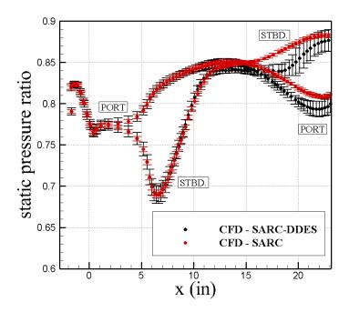
**Figure 11.** Unsteadiness in solutions of M2129 intake. Dot markers show time-averaged static to free-stream total pressure value of the NASA baseline grid. Bar denotes maximum difference from averaged values. Static pressure ratio ( $p_f/p_{0\infty}$ ) is the ratio of averaged engine face static pressure to free-stream total pressure.
