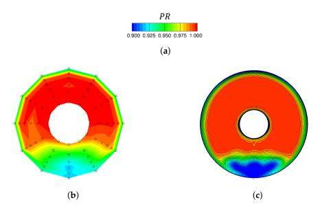
**Figure 6.** Experimental and simulated engine face pressure ratio. NASA grid was used with SARC-DDES turbulence model. CFD data are time-averaged from 2 to 2.5 s of simulation time. (a) Pressure recovery range; (b) Experimental data; (c) CFD—Baseline.
