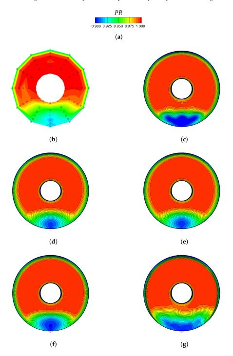
Figure 9. Effects of turbulence model on engine face pressure ratio. Time-averaged solutions are shown for the NASA baseline grid. (a) Pressure recovery range; (b) Experimental data; (c) CFD–SARC + DDES;
