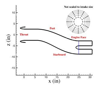
**Figure 1.** The sketch of the RAE M2129 geometry used in this work. The pressure rakes at the engine face are shown as well. They include 12 equally spaced arms with 30-degree intervals with six pitot pressure probes at each arm.
