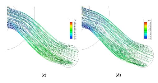
**Figure 13.** Streamlines colored by pressure coefficient. NASA baseline grid was used. CFD data are time-averaged from 2 to 2.5 s of simulation time. (a) SARC turbulence model; (b) SARC + DDES turbulence model; (c) SST turbulence model; (d) SST + DDES turbulence model.
