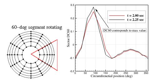
**Figure 7.** Illustration of the DC60 calculation approach. In the left, a 60-degree segment is shown which is at zero circumferential angle. The sector rotates clockwise one degree at a time. In the right, DC60 values for the 60-degree segment at each angle are shown. These plots correspond to simulation times of 2 and 2.25 s.
