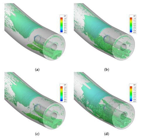
**Figure 12.** Isosurfaces of scale Q-criterion (iso value of 0.25) colored by pressure coefficient. NASA baseline grid was used. CFD data are time-averaged from 2 to 2.5 s of simulation time. (**a**) SARC turbulence model; (**b**) SARC + DDES turbulence model; (**c**) SST turbulence model; (**d**) SST + DDES turbulence model.
