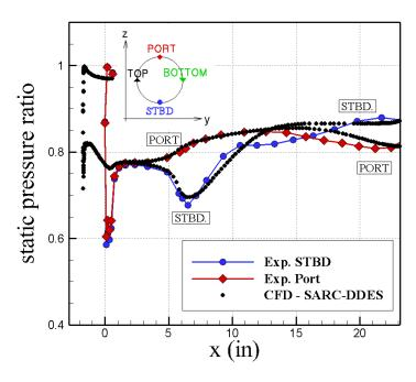
**Figure 8.** M2129 DP78 wall pressure measurements and simulations using Kestrel and SARC–DDES turbulence model. Static pressure ratio,  $p_f / p_{0\infty}$ , is the ratio of averaged engine face static pressure to free-stream total pressure. NASA baseline grid was used. CFD data are time-averaged from 2 to 2.5 s of simulation time.
