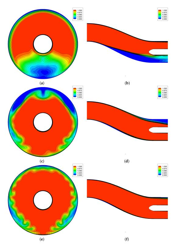
**Figure 14.** Engine face and symmetry pressure ratio using USAFA grids and SARC-DDES turbulence models. CFD data are time-averaged from 2 to 2.5 s of simulation time. (a) Baseline engine face; (b) Baseline symmetry; (c) Baseline + VG engine face; (d) Baseline + VG symmetry; (e) Baseline + Jets engine face; (f) Baseline + Jets symmetry.
