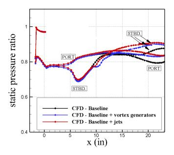
**Figure 15.** Wall pressure data for the baseline, baseline + vortex generators, and baseline + jets simulations. Static pressure ratio ( $p_f/p_{0\infty}$ ) is the ratio of averaged engine face static pressure to free-stream total pressure. USAFA grids and SARC-DDES turbulence models were used. CFD data are time-averaged from 2 to 2.5 s of simulation time.
