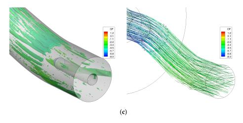
**Figure 16.** Isosurfaces of scale Q-criterion (iso value of 0.25) and streamlines colored by pressure coefficient. USAFA grids and SARC-DDES turbulence models were used. CFD data are time-averaged from 2 to 2.5 s of simulation time. (a) Baseline; (b) Baseline + VG; (c) Baseline + Jets.
