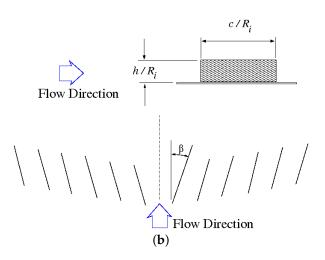
**Figure 2.** The RAE M2129 vortex generator locations and geometry parameters. These pictures were adapted from Ref. [12]. (a) VG locations; (b) Geometric parameters.
