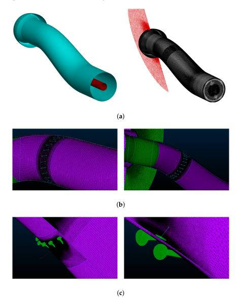
**Figure 4.** USAFA baseline intake model with vortex generator plates and jets. (**a**) USAFA baseline geometry and symmetry grid; (**b**) Vortex generator plates; (**c**) Jets.
