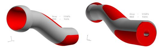
**Figure 3.** RAE M2129 geometries. NASA model was obtained from Bernhard Anderson. USAFA model was created from given intake data and offset and diameter changes equation with length.
