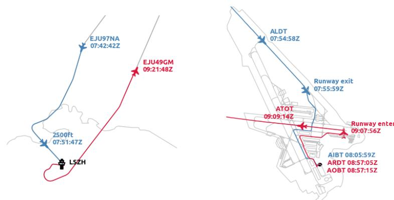
**Figure 1.** ADS-B-based milestone approach for data-driven operational awareness and framework for upcoming prediction tasks using Zurich Airport (LSZH) as an example [37]. Milestones are for instance actual in-block time (AIBT), aircraft ready time (ARDT), actual off-block time (AOBT), or actual take-off time (ATOT).
