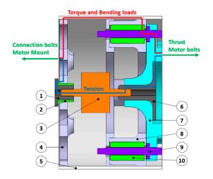
tension rod (traction stop) friction bearing tension sensor connecting frame housing force introduction bolt engine connection plate load transmission frame linear guide pins linear bearing
