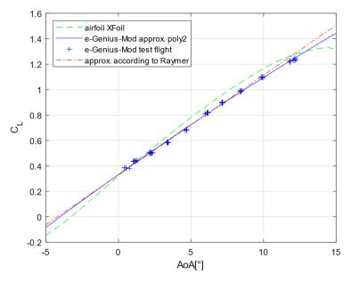
Figure 14. Comparison of XFoil airfoil simulation, semi empirical method and flight test data.
