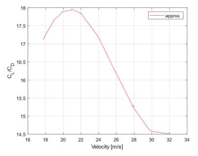
**Figure 11.** Glide ratio  $(C_L/C_D)$  to velocity.
