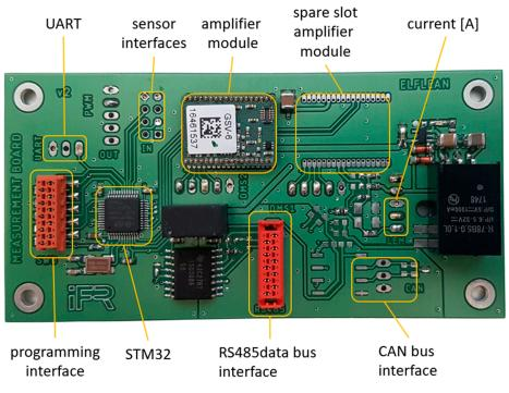
Figure 5. Data Acquisition Unit.
