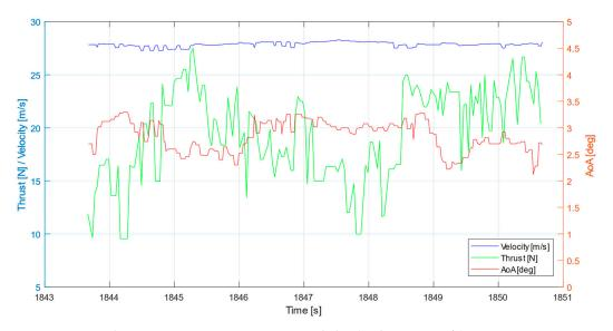
Figure 8. Example: Basic measurements on one single leg (with TAS 28 m/s).
