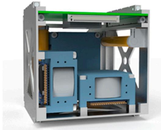
**Figure 12.** Swappable ADCS box accommodating control electronics and actuators.
