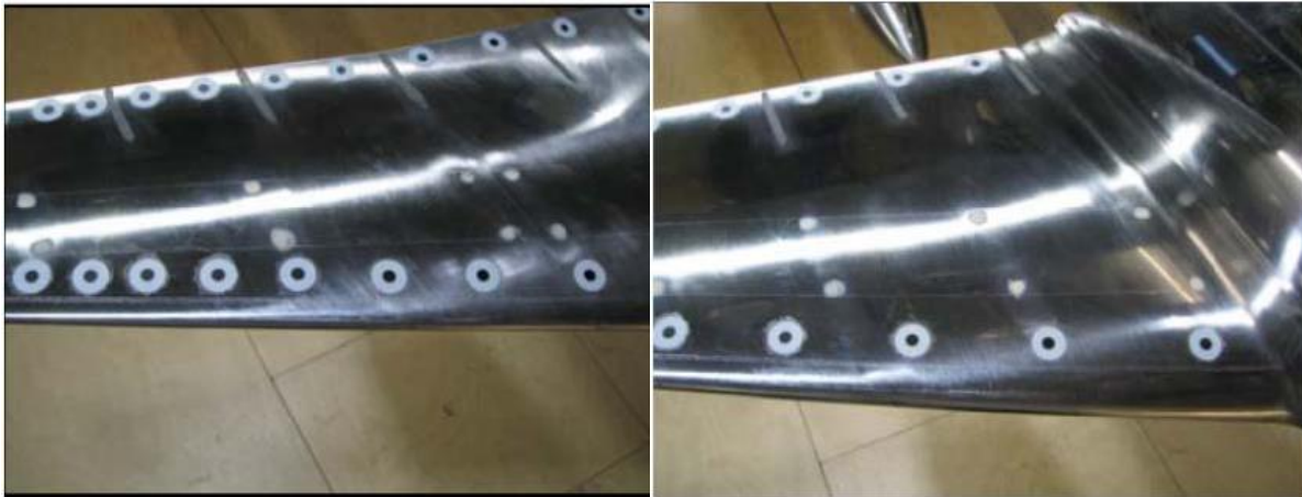
Figure 3. SPT markers on the supercritical wing.
