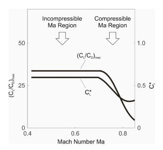
**Figure 5.** Maximum lift-to-drag ratio,  $(C_L/C_D)_{max}$  and associated lift coefficient,  $C_L^*$ , dependent on Mach number, Ma, (relating to drag polar in Figure 4.
