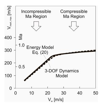
**Figure 9.** Maximum speed,  $V_{inert,max}$ , dependent on wind speed,  $V_w$ .
