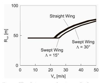
**Figure 19.** Effect of wing sweep on the trajectory radius for swept wing configuration 1 in maximum-speed dynamic soaring.
