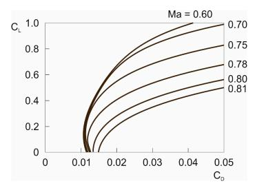
**Figure 4.** Drag coefficient of straight wing configuration dependent on lift coefficient,  $C_L$  and Mach number, Ma, [7].
