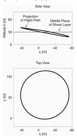
**Figure 7.** Side and top views of dynamic soaring loop optimized for maximum speed,  $V_{inert,max} = 271.8 \text{ m/s}.$
