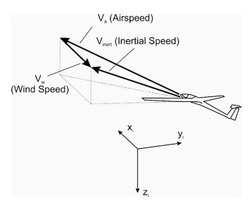
**Figure 2.** Speed vectors and inertial coordinate system. (The x axis is chosen parallel to the wind speed vector  $V_w$  and pointing in the opposite direction).
