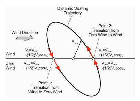
**Figure 3.** Oblique view on high-speed dynamic soaring loop. (The inclination of the trajectory relative to the horizontal is shown exaggerated for representation purposes).
