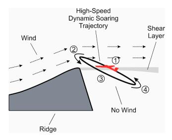
Figure 1. High-speed dynamic soaring trajectory and shear wind scenario at ridge.
