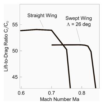
Figure 12. Effect of Mach number, Ma, on lift-to-drag ratio of glider model wings (from [23]).
