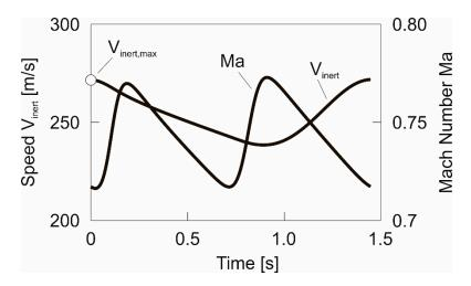
**Figure 8.** Time histories of speeds,  $V_{inert}$  and  $V_a$ , and Mach number, Ma, of dynamic soaring loop optimized for maximum speed,  $V_{inert,max} = 271.8 \text{ m/s}$ .
