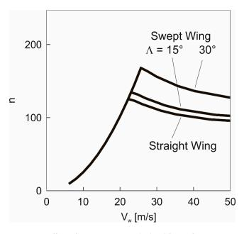
**Figure 18.** Effect of wing sweep on the load factor for swept wing configuration 1 in maximum-speed dynamic soaring.
