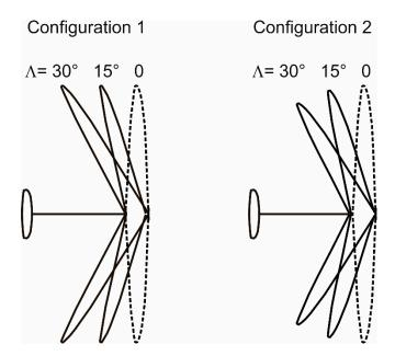
Figure 14. Swept wing configurations 1 and 2.
