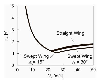
**Figure 17.** Effect of wing sweep on the cycle time for swept wing configuration 1 in maximum-speed dynamic soaring.
