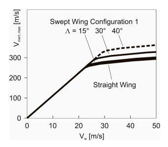
**Figure 15.** Effect of wing sweep on maximum speed,  $V_{inert,max}$ , for swept wing configuration 1.
