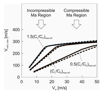
**Figure 11.** Maximum speed,  $V_{inert,max}$ , dependent on wind speed,  $V_w$  and on maximum lift-to-drag ratio,  $(C_L/C_D)_{max}$ . Results obtained using the energy model, Equation (20).
