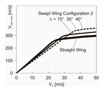
**Figure 16.** Effect of wing sweep on maximum speed,  $V_{inert,max}$ , for swept wing configuration 2.
