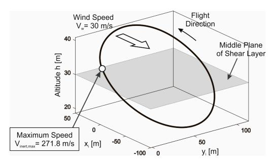
**Figure 6.** Dynamic soaring loop optimized for maximum speed,  $V_{inert,max} = 271.8 \text{ m/s}$ .
