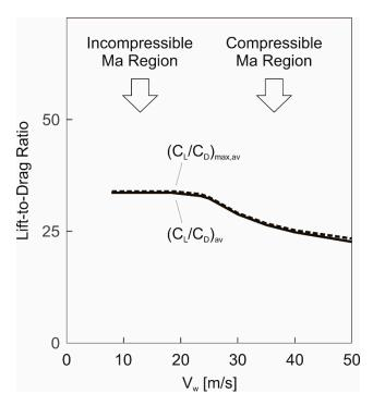
**Figure 10.** Lift-to-drag ratio in maximum-speed dynamic soaring.  $(C_L/C_D)_{av}$ : actual lift-to-drag ratio, 3-DOF dynamics model;  $(C_L/C_D)_{max,av}$ : maximum lift-to-drag ratio, 3-DOF dynamics model.
