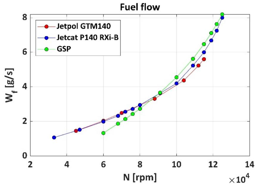
Figure 9. Fuel flow compared with GSP model.
