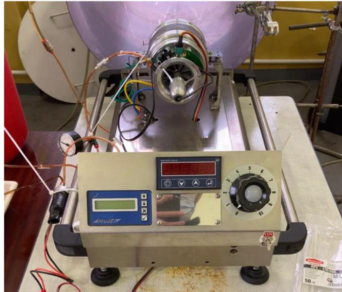
Figure 1. JETPOL GTM 140 at the test rig.
