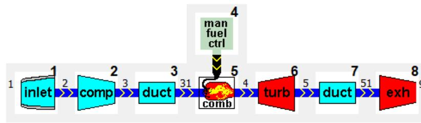
Figure 8. Engine model in GSP.
