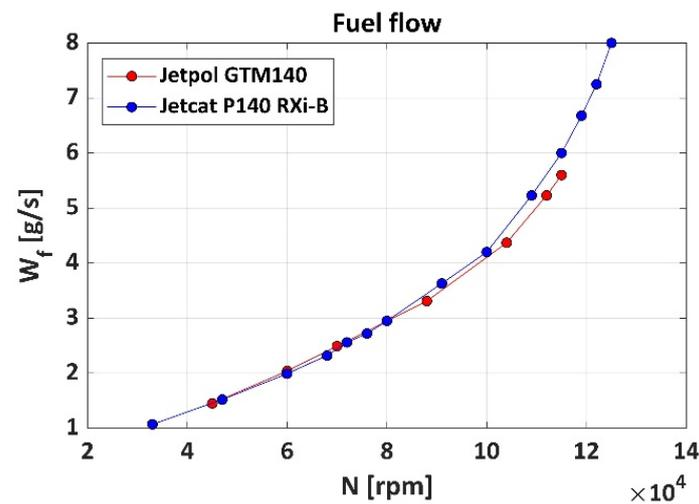
Figure 2. Fuel flow vs. rotational speed.
