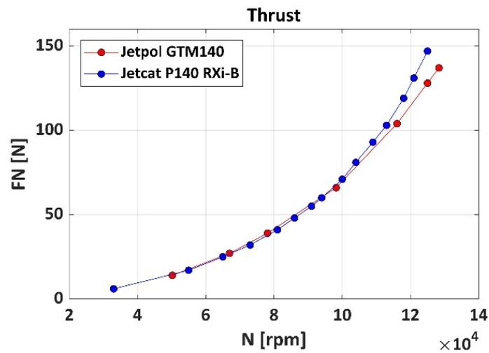
Figure 3. Thrust vs. rotational speed.
