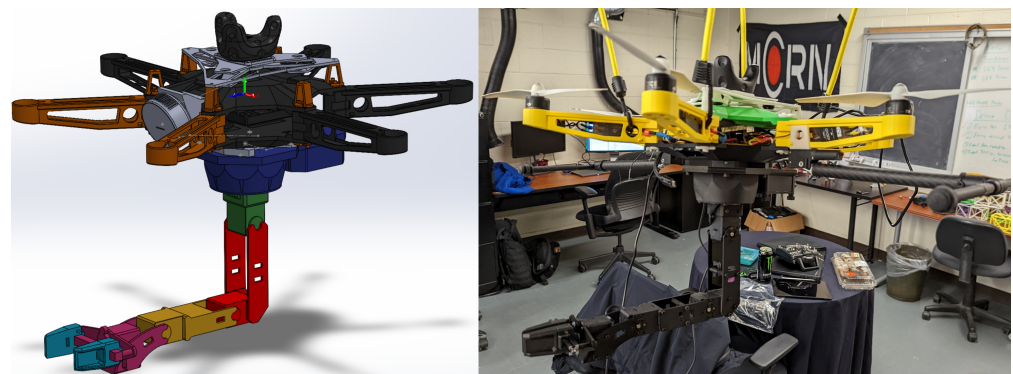
Figure 23. Depiction of the integrated drone, camera, and robotic arm system.
