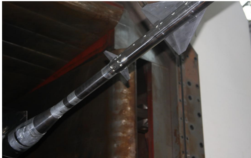
Figure 7. Support sting in wind tunnel test.
