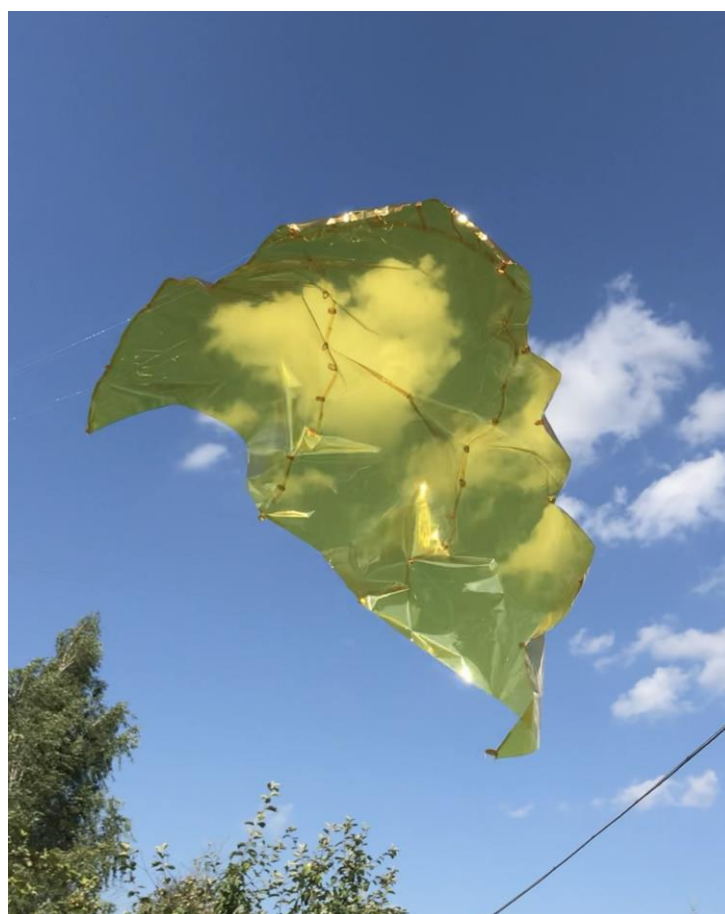
Figure 12. Prototype Kapton wing being flight-tested as a kite.
