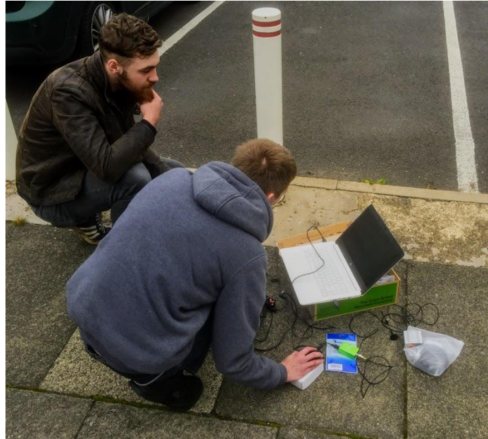
Figure 22. Setting up the ground station, with ThumbNet “N3” SDR receiver (green) to lower right.
