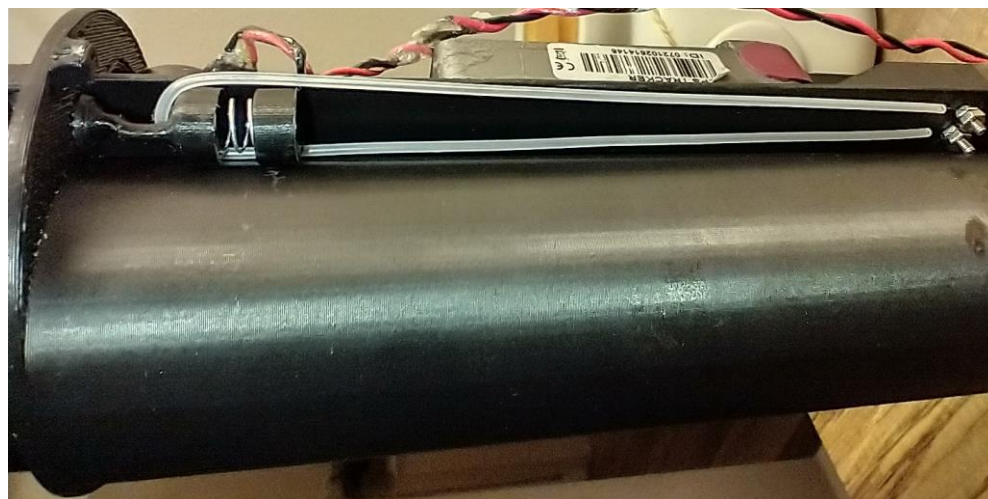
Figure 16. Shape memory alloy wire with silicone sheath.
