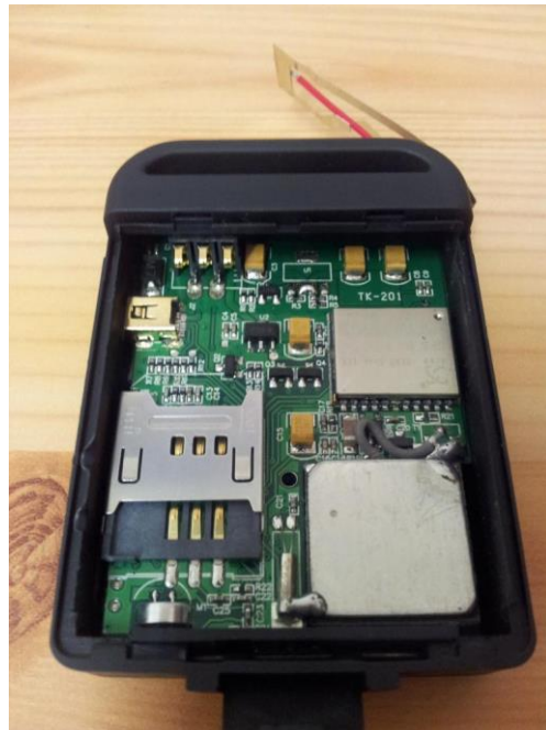
Figure 15. TK102B GPS/GSM tracker module—antenna at top.
