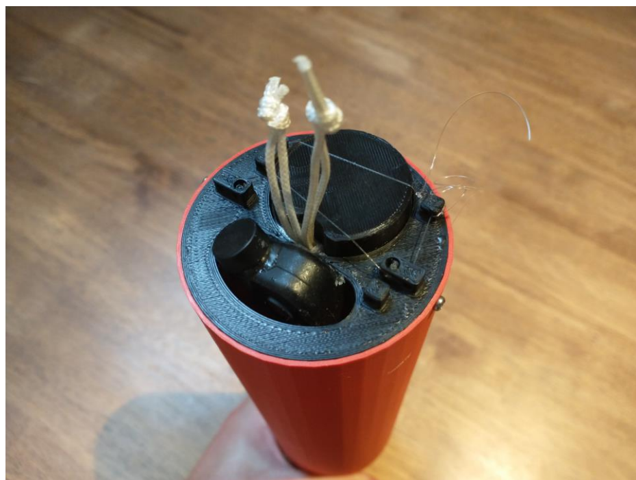
Figure 17. Rear of capsule, with circular parawing container “cap” at top, pinpuller lugs at right and left.
