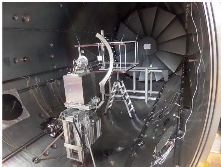
Figure 9. View of the experimental setup in the STG-ET chamber: thruster, hanging coils, and LDBS system behind the ladder are visible.
