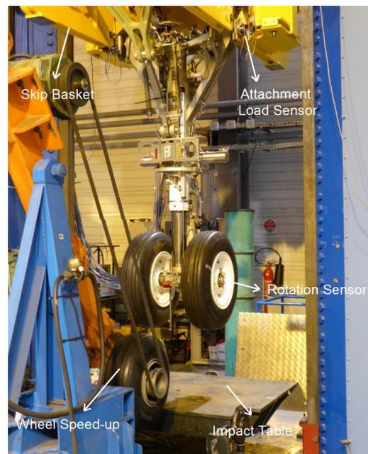
**Figure 7.** Landing gear drop test facility.
