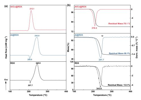
Figure 4. The (a) DSC and (b) TG-DTG curves for the studied Al/Co-based composites.
