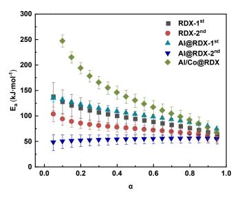
**Figure 6.** Activation energies vary as a function of the conversion degree obtained for both RDX and the corresponding RDX composites.
