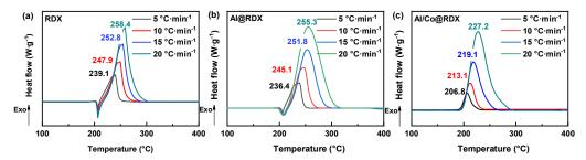
Figure 5. The DSC curves for (a) RDX, (b) Al@RDX and (c) Al/Co@RDX at different heating rates.
