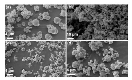
**Figure 2.** SEM micrographs of the powders involved in this study: (a) Al, (b) Co, (c) Al/Co and (d) Al/Co@RDX.
