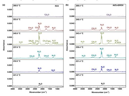
Figure 8. Compiled FTIR spectra recorded for (a) pure RDX and (b) Al/Co@RDX.
