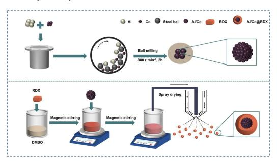
Figure 1. Schematic illustration of the preparation process of the Al/Co@RDX composite.
