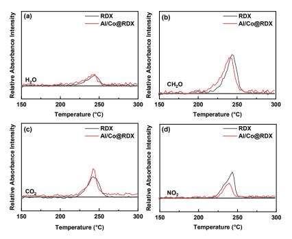
**Figure 9.** Comparison of the temperature-dependent relative gas absorption intensity between RDX and Al/Co@RDX for: (a)  $H_2O$ , (b)  $CH_2O$ , (c)  $CO_2$  and (d)  $NO_2$ .
