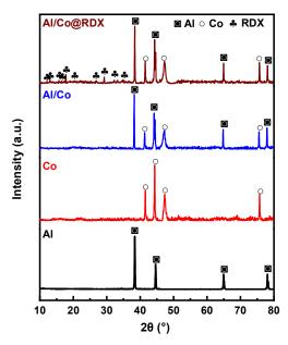
Figure 3. The XRD diffraction peaks of the raw materials and the Al/Co@RDX composite.
